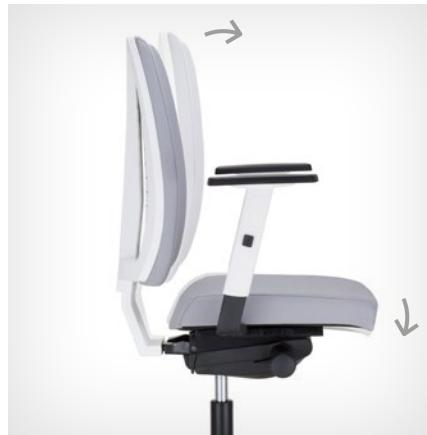
Seat negative angle of  $3^\circ$  tilting with the backrest at  $6^\circ$  allows for chair tilting and eliminates the unfavourable effect of raising knees at the same time. The function is particularly useful when it comes to typing on the keyboard.
